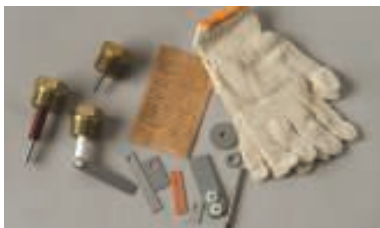
FIGURE 1. Weight-loss coupons are installed for a period, then weighed to determine corrosion
