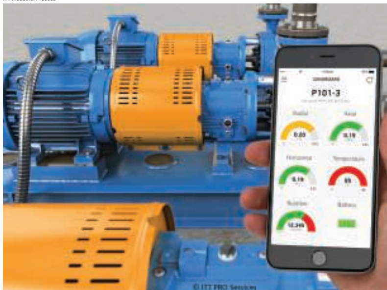
FIGURE 4. ITT Industrial Process's i-Alert2 equipment health monitor, a Bluetooth smart device, tracks vibration, temperature and run-time hours, trends information and has the ability to diagnose machine faults with vibration and other analysis tools and can send alarms if equipment is outside normal operating conditions
