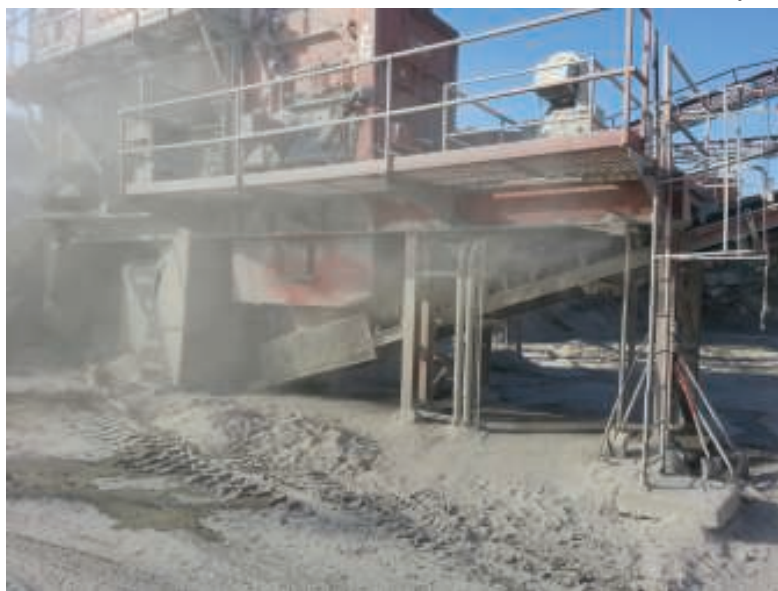
FIGURE 2. Loading and unloading points for solids can present significant dust control challenges
