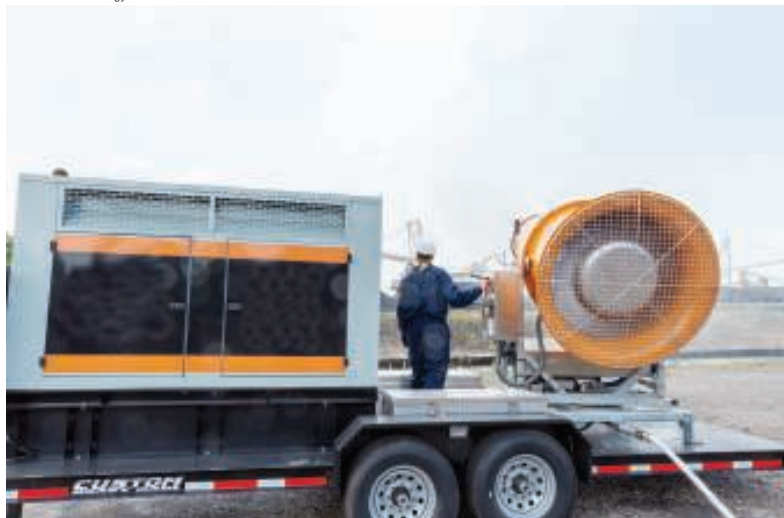
FIGURE 12. This atomized mist design employs a 60-hp fan and a high-pressure booster pump
