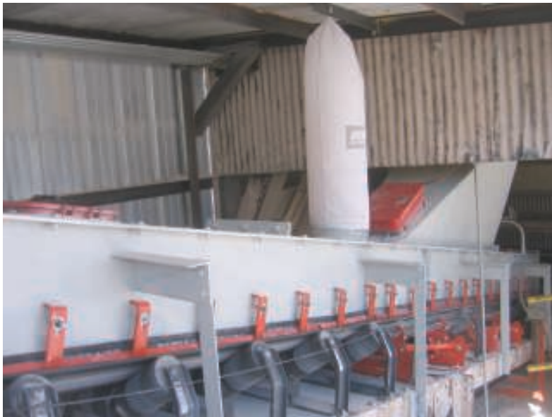
FIGURE 4. Dust bags filter outgoing air to minimize fugitive material, while reducing positive air pressure
