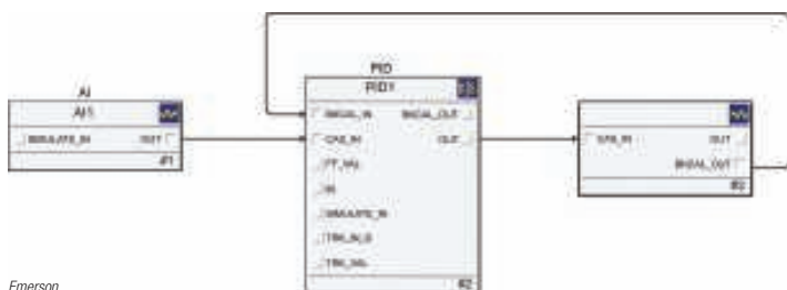
FIGURE 8. When control is accomplished in the control system, additional delay is introduced because control actions are not synchronized with fieldbus processing
