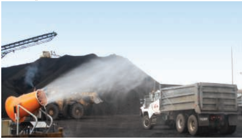
FIGURE 11. Atomized mist is one of the few techniques able to control both surface dust and airborne particulate matter
