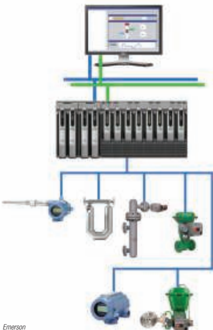
FIGURE 5. Fieldbus is a digital communication system allowing multiple devices to connect on a segment. Redundancy options decrease failure points and improve integrity
